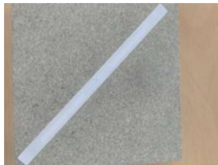
Etiqueta A - WET INLAY UHF H3 96/512B 124x7 mm
